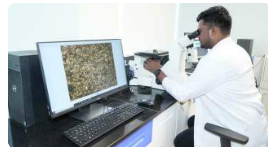
Dadri R&D Centre, Testing Micro Structure of Wire.
