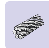
Steel Rope Wires
